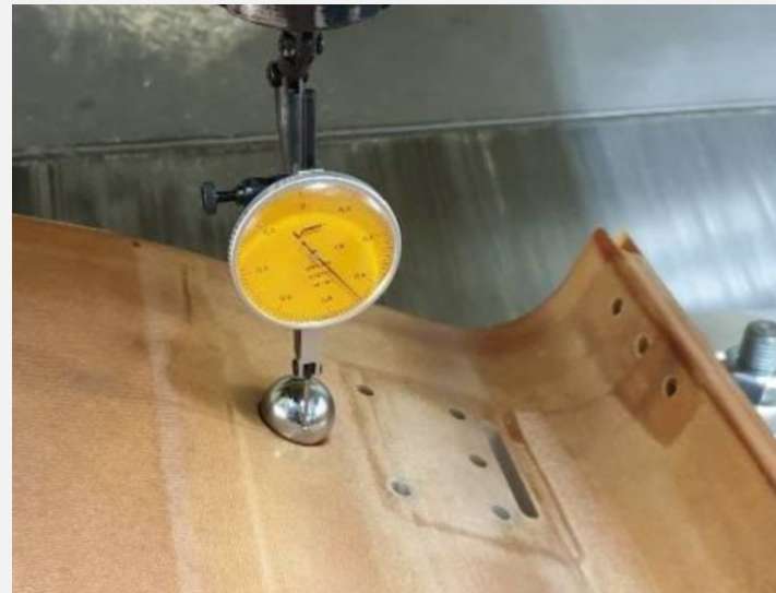
Moulded Machining Datum positioning
