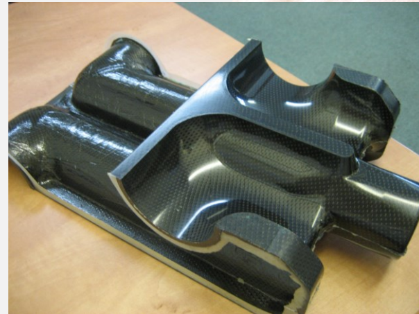
Structural attachments: Tongue and Groove Assembly with I-ply detail
