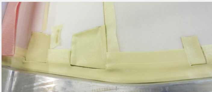
Embedded ply-stacked hardpoints
